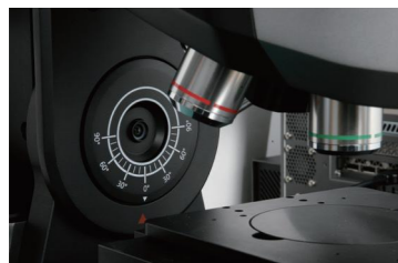
side camera shows the relationship between the lens and the workpiece, reducing the risk of collision
